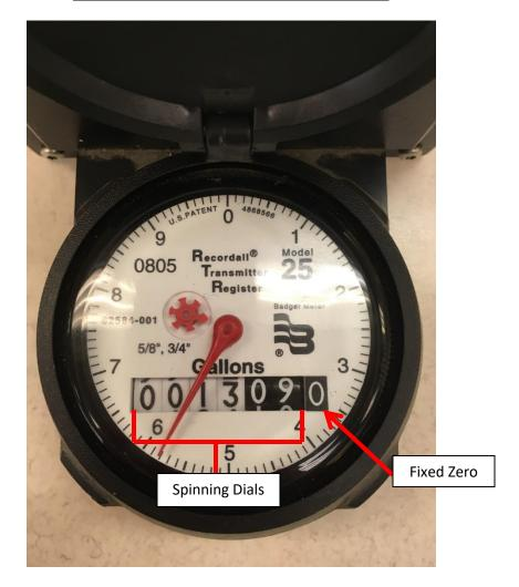
Look at the spinning dials on your meter. The above meter would show on your bill as Current Meter Reading "1309." The difference of the two reads on your bill will be multiplied by 10 to account for the fixed zero on the meter.
