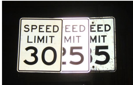
Figure 13: Retro-reflectivity of a speed limit sign
