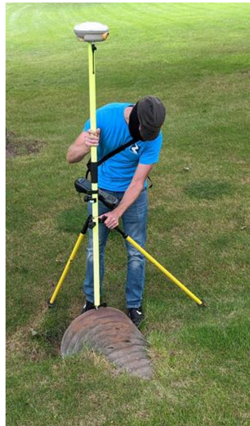
Figure 3. FW surveyor collecting culvert invert elevation data.
